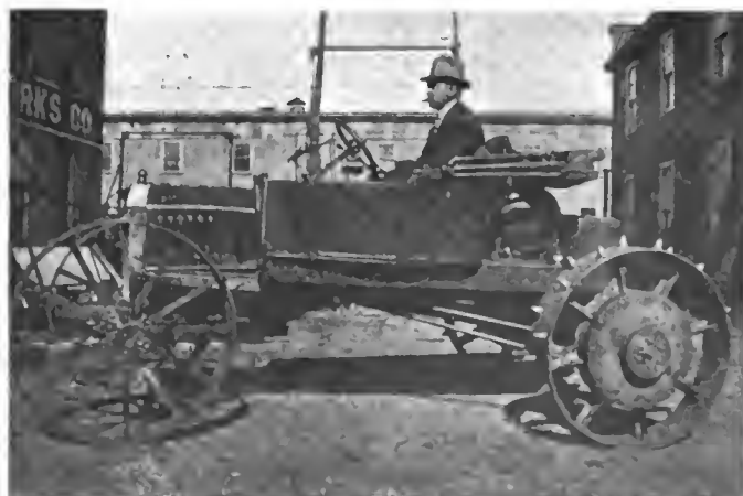
Left—Megow tractor attachment on a Ford roadster and drawing two 14-in. stubble plows. Note deep furrows and also plowed area to the right of the machine. At the right the same vehicle, in side view, gives an idea of the type of wheels used for tractor purposes
